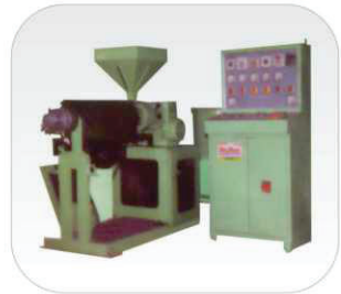
Pvc Codun Pipe Plant
