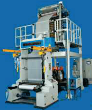
ABA Co-Extrusion Film Plant
