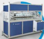
Tube/Pipe - Traction Unit
