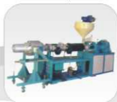
HDPE Pipe Plant
