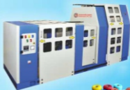
▶ HIGH SPEED ROPE MAKING MACHINE 2mm To 6mm
