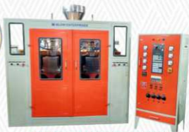
2 LTRS. DOUBLE STATION / 4 CAVITY WITH AUTO DE-FLASHING ATTACHMENT
