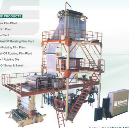
THREE LAYER FILM PLANT
