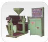
Pvc Codun Pipe Plant
